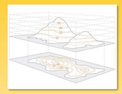
A contour is a line drawn on a map that joins points of equal height above sea level.
